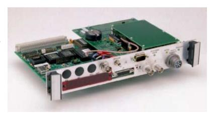
The VME-SyncClock32 with P(Y) code receiver from Brandy-wine Communications provides precision time to the host computer over the VME bus with zero latency. The on-board microprocessor automatically synchronizes the clock to the input reference signal. The reference signal inputs can be GPS, 1 PPS or time codes. The 1PPS or time code inputs will become the reference input should the GPS input fail. The clock can free run and be set by commands from the host over the VME bus.
